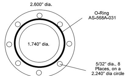
For mounting a vessel to the unit.
