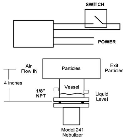
A typical set-up is shown for generating fine particles and carrying them off for processing. Optimum height for 2 cfm air flow is 4"
