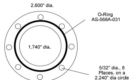
For mounting a vessel to the unit.
